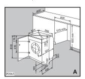
When installing the appliance into the kitchen furniture ensure, if possible, the hoses are placed in either of the two recesses on the back of the appliance.
